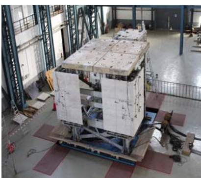
Facade system Natural stone - Moucharabieh Seismic qualification testing of facade system of Djamaâ El-Djazair
