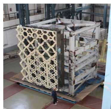
Facade system Natural stone - Moucharabieh Seismic qualification testing of facade system of Djamaâ El-Djazair
