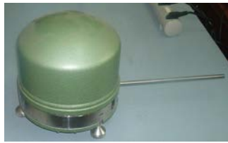
Station sismologique large-bande (STS2+Q330+Baler)
